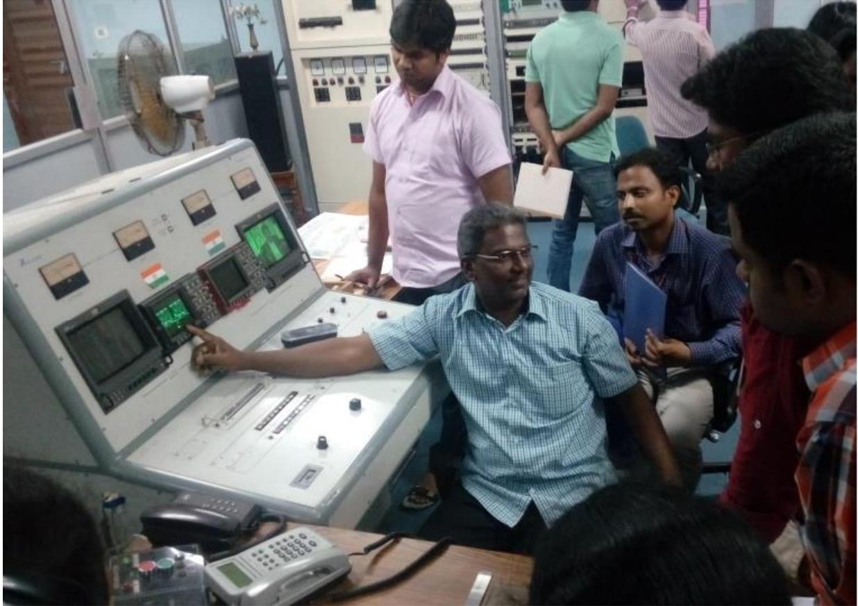
During the technical session the resource person explained about visualization of TV signal, color carrier , sync pulse timings and how color video is transmitted using the existing monochrome television system
